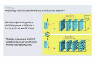
The local increase of concentration in front of the solidif cation front leads to a reduction of the liquidus temperature compared to the phase diagram: The melting undercools (constitutional undercooling). The higher the undercooling, the higher the instability of the crystal growth front. The actual temperature in front of the solidif cation front depends on the temperature gradient.
